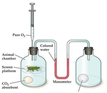
Inert object that occupies a volume equal to the volume occupied by the animal and the CO<sub>2</sub> absorbent in the animal chamber
