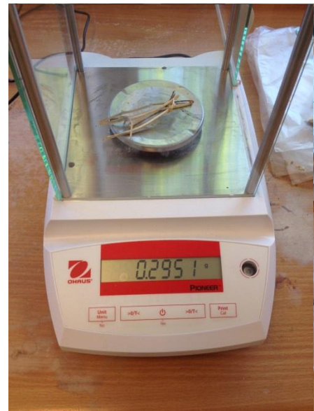
Picture 2.9 shows how dry weight was measured.
