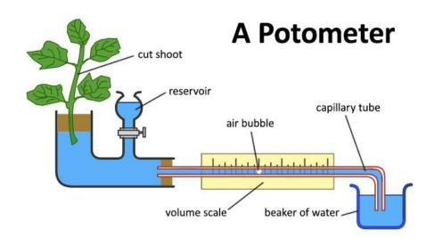
This is basically a device to measure how fast the water uptake is by movement of bubble. Since water is lost by transpiration, air bubble will move towards the plant. Reservoir is to remove the air bubble so new trials can be made.
